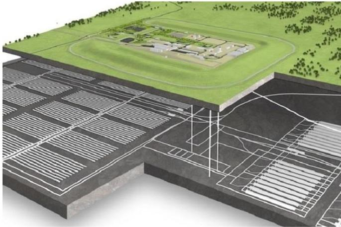
Figure 1. Schematic representing a deep geological disposal facility for higher activity radioactive wastes. ([www.gov.uk](http://www.gov.uk))
